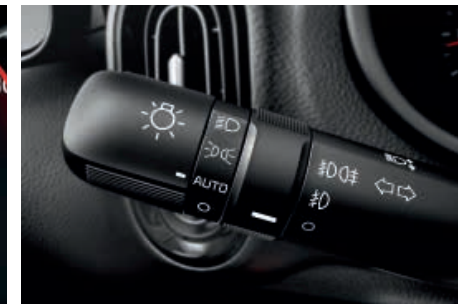
Auto light control Set the stalk ring to Auto and the front and rear lights will turn on or off depending on lighting conditions.
