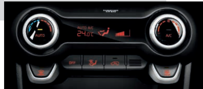
Auto Temperature Control Enjoy one-touch comfort with Auto Temperature Control. Just set your preferred temperature, and the automatic system will monitor and maintain it until you change or cancel the setting.
