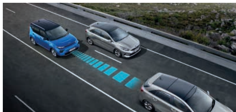
Smart Cruise Control. Using a camera and radar sensor at the front, this functionality regulates your speed based on a set speed and the desired distance to the vehicle ahead. If the vehicle ahead picks up the pace, the Soul EV accelerates up to the set speed. If the vehicle in front slows down and the predetermined safe distance cannot be maintained, the system reduces the speed, or even stops the car. A helpful feature on the motorway and in stop-and-go traffic.
