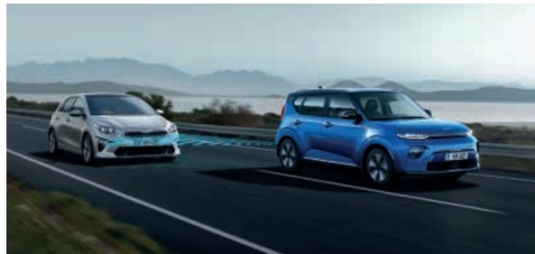
Blind-Spot Collision Warning. The Blind-Spot Collision Warning system has radar sensors that monitor your blind spots and vehicles attempting to overtake. Your door mirror displays a symbol if a vehicle is detected. The system also sounds an audible alert if you indicate while a vehicle is present.
