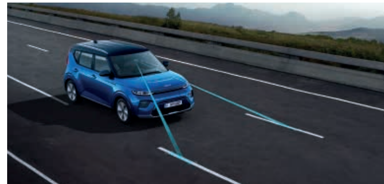
Lane-Keeping Assist and Driver Attention Warning. These systems help prevent risks associated with sleepiness at the wheel. Lane Keeping Assist warns you and steers you back in your lane if you are drifting out of it. Driver Attention Warning continuously assesses your driving and asks you to take a break when it senses your level of attention is flagging.
