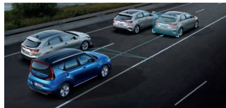
Lane Follow Assist. Very useful for motorway driving, Lane Follow Assist monitors road markings to keep your car in the centre of your lane.
