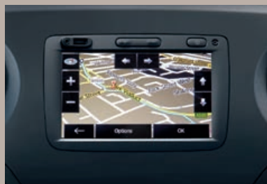
Dynamic satellite navigation* IntelliLink infotainment system with 7-inch colour touch-screen facility.
