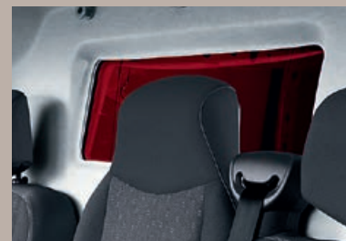
Bulkhead window A window for the steel bulkhead is available as an option, protecting the driver and crew while allowing an uninterrupted view of the cargo bay.
