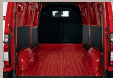
Load area protective panels Half-height load trim panels help safeguard the side walls from everyday wear and tear. Standard on RWD models.
