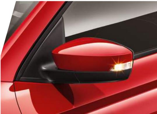
ELECTRICALLY ADJUSTABLE AND HEATED DOOR MIRRORS
