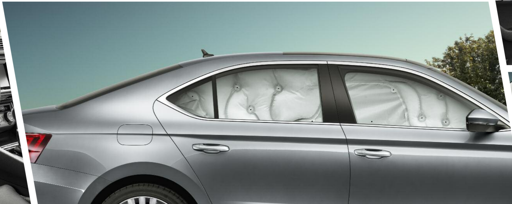
The front and rear side airbags protect the pelvis and chest of the driver and other passengers in the event of a side collision.
