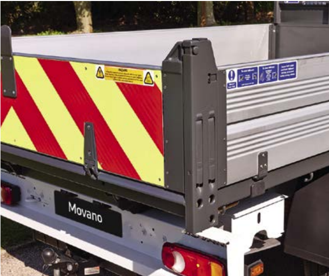
Locking handles enable quick and safe full dropside capability.
