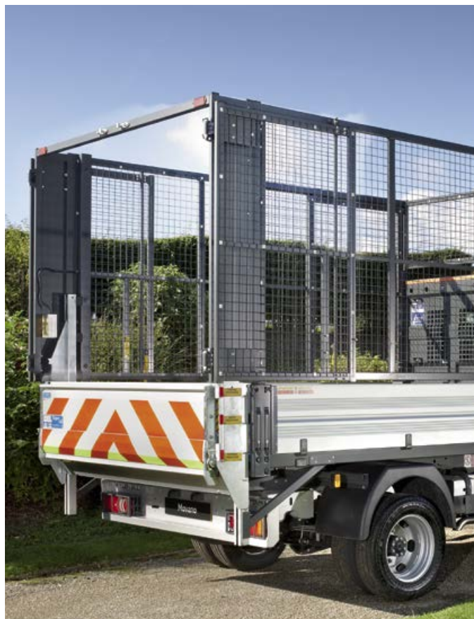
270° opening/lockable rear doors. The 500kg tail lift (illustrated), is optional at extra cost.
