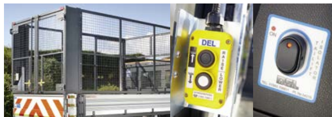
The tipper can be operated from the cab or via a spiral wander-lead. Isolator switch for tail lift function.
