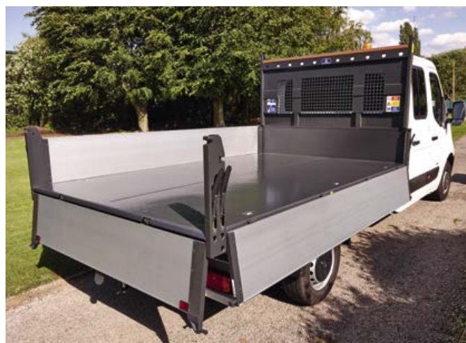
The Utility Cab Tipper conversion also features full dropside capability.
