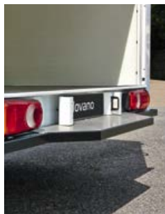
Low rear step height – 400mm.
