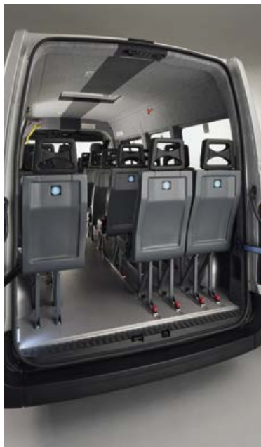
Four of the rear seats feature quick-release fixings for easy removal providing loadspace or to create space for two wheelchair passengers.
