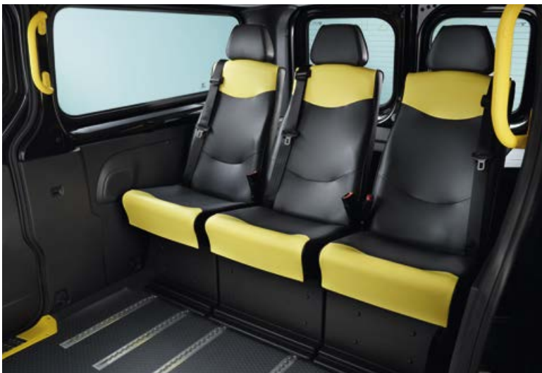
The three rear seats are mounted on quick-release tracking.
